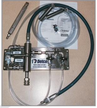
the wand. This causes internal wear and premature damage to the coil, pump seals, packing and o-rings. The D-522 Airless Bypass Foamer allows the chemical to be injected just before the wand bypassing the pump and coil. This will increase the life of the pump and coil.
